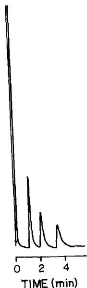
Fig. 2. Separation of C_{36} , C_{38} and C_{40} n -alkanes on a 1\text{ m} \times 2\text{ mm} I.D. glass column packed with 10% (w/w) Fomblin YR on Chromosorb P (100-120 mesh), temperature 255^\circ\text{C} , nitrogen carrier gas flow 20\text{ ml min}^{-1} .
